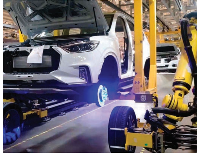
Advanced robotic guidance solution utilizing Unblink3D Robotics 3D Vision Toolbox to automate wheel installation.
